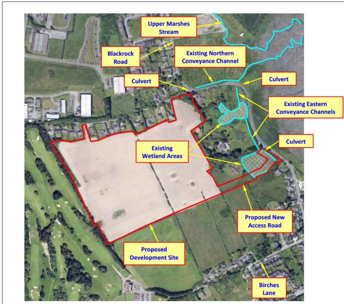
Figure 10.3 - Local Offsite Drainage Channels and Wetland Areas Located Downgradient of the Site.
